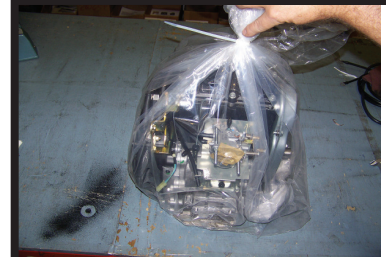
Install Engine In Plastic Bag
